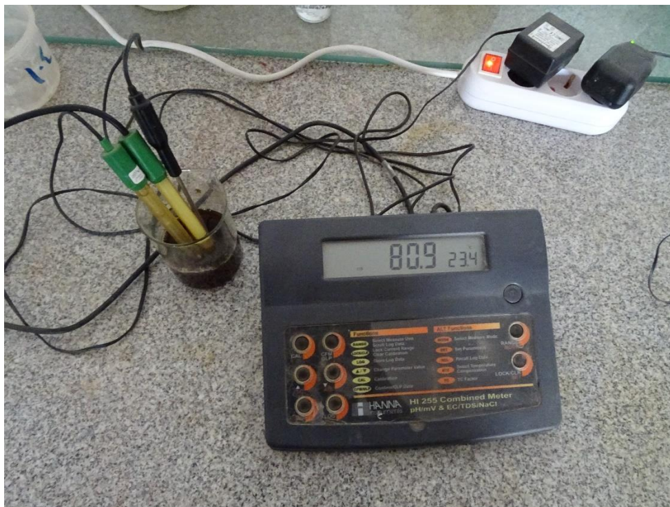
Figure 3. 4: Combined pH/mV and EC/TDS/NaCl meter used during the experiments
