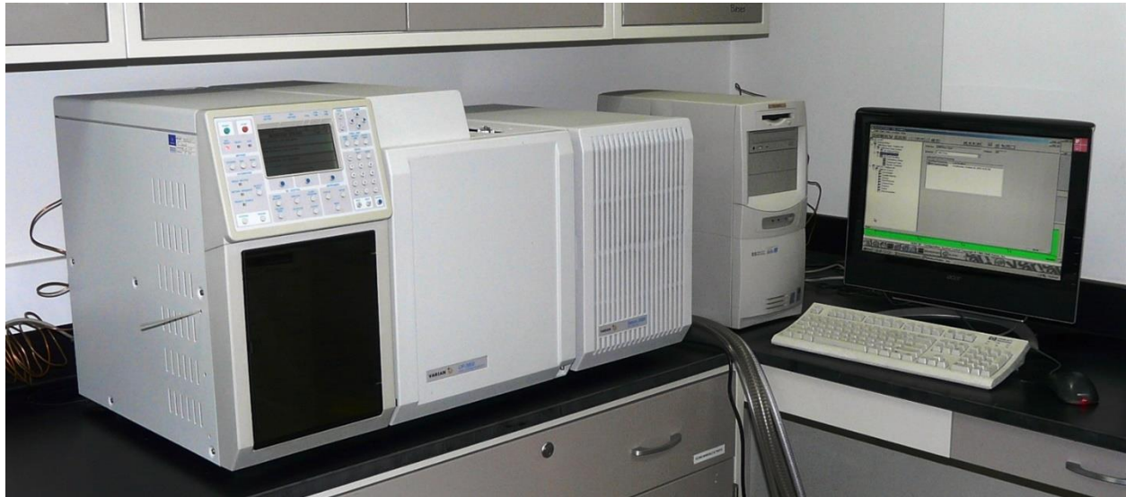
Figure 3. 5: Varian CP 3800 chromatograph used in the chemical analysis of biogas samples
